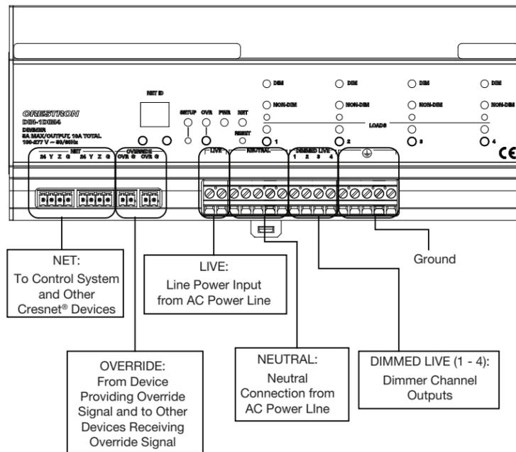
With the circuit breaker turned off, connect the wires to the terminal blocks per the markings provided on the DIN-1DIM4.
