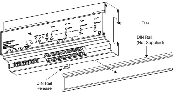
**Remove the DIN-1DIM4**
