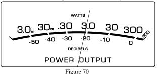
The meters respond to all the musical information being produced by the Amplifier. They indicate to an accuracy of at least 95% of the power output with only a single cycle of a 2,000Hz tone burst.
