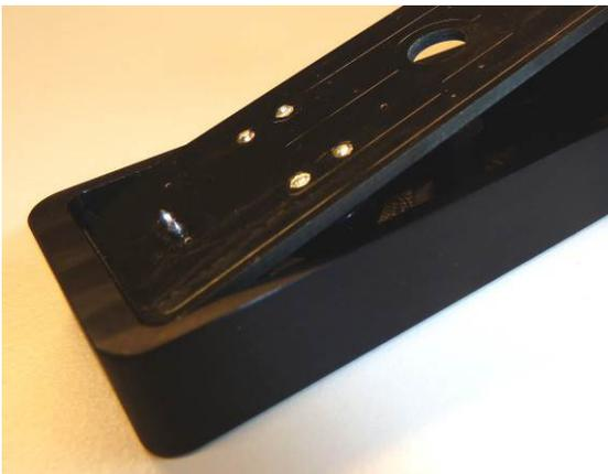
When the new battery is placed, lay back this part of the board where the blue led is situated. The led will be positioned in front of the recess. Next you can lay down the whole board in the housing. Next you can place the cover and tighten the screw.
