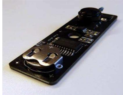
By turning the housing upside down the printed circuit board will fall out and the component side will be visible now.
