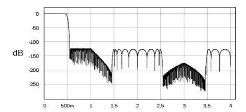
The Fast (Linear Phase) filter is a highly regarded audio filter offering low ripple in both the pass and stop bands, and what is known as constant group delay. Constant group delay means that audio signals of all frequencies are always delayed by the same amount when passing through the filter. All audio is therefore fully time-coherent at the output.
