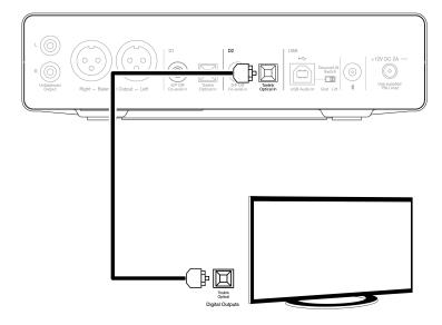
**Important Note:** Only connect one co-axial OR optical cable to each digital input. The unit will not operate properly if both connections are made (even if only one is active).
