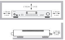
WARNING: The rear panel power cord connector is the mains power disconnect device. The device must be located in an open area that allows access to the cord connector.
