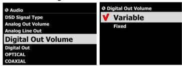
You can set Analog Out Volume as Variable or Fixed X Default: Variable Fixed: N25AMP volume will be set as OdB (Max). You can't control volume with N25AMP
