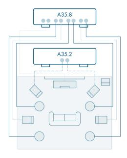
Adds an A35.2 stereo amplifier for the Front Left and Right speakers, while using one bridged pair of outputs from the A35.8 for Centre, and the remaining outputs from the A35.8 for Surround Left and Right, Front Height Left and Right, and Rear Height Left and Right speakers.
