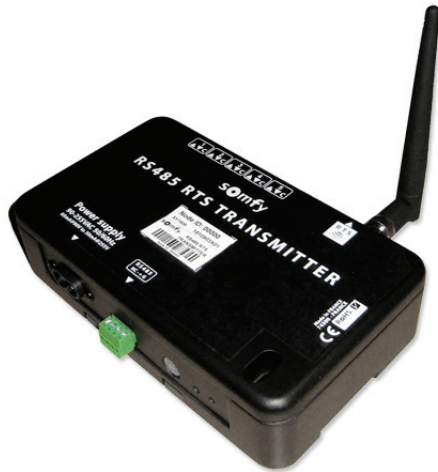
RS485RTS transmitter Surface or DIN rail mounting wireless motor controller Accessories: Aerial extension kit (PN 9015314)
