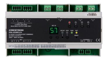
**Dim Load Types:** 0-10 Volt fluorescent ballast or LED driver (4-wire); Maximum of 30 dimmable ballasts/drivers
